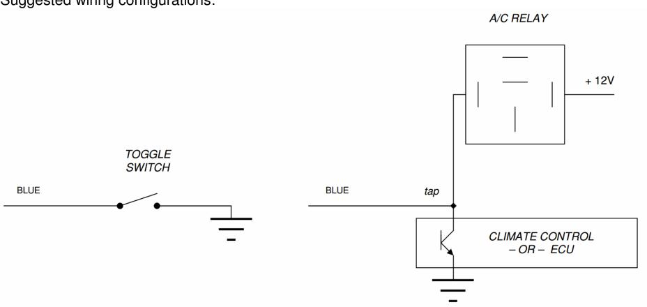
Note: If using a manual override switch with the low speed and high speed inputs it is suggested that they be grounded back to the same ground source as the module. In some instances, if there is a significant difference in the ground voltage from the module to the ground of the switch, the controller may not activate the fans correctly.
